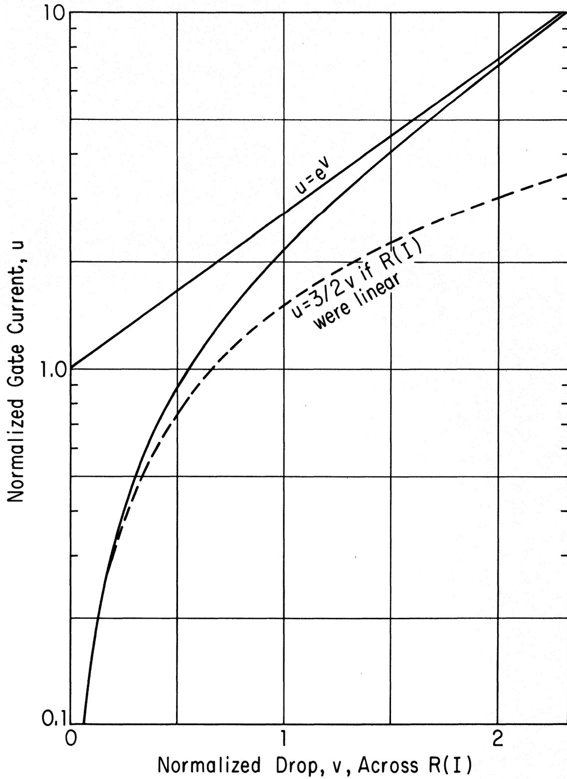
Figure 2. The volt-ampere characteristic of  $R(I)$ .
