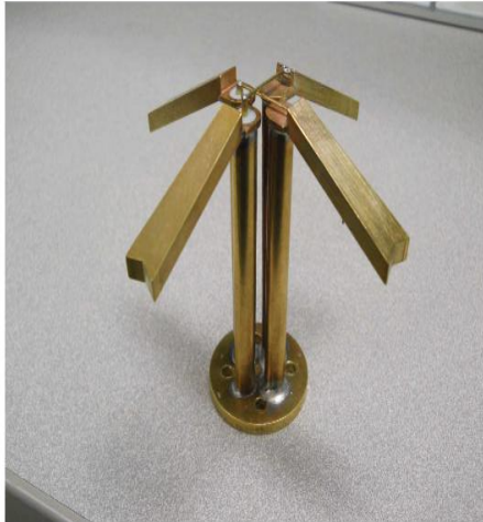
Figure 2: Left: Dual-pol phased array element “kite” design matched to cryogenic low noise amplifiers. Right: L-band phased array feed cryostat (R. Norrod, NRAO).
