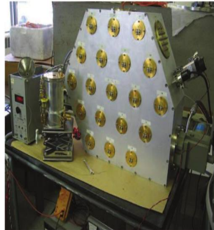
Figure 2: Left: Dual-pol phased array element “kite” design matched to cryogenic low noise amplifiers. Right: L-band phased array feed cryostat (R. Norrod, NRAO).
