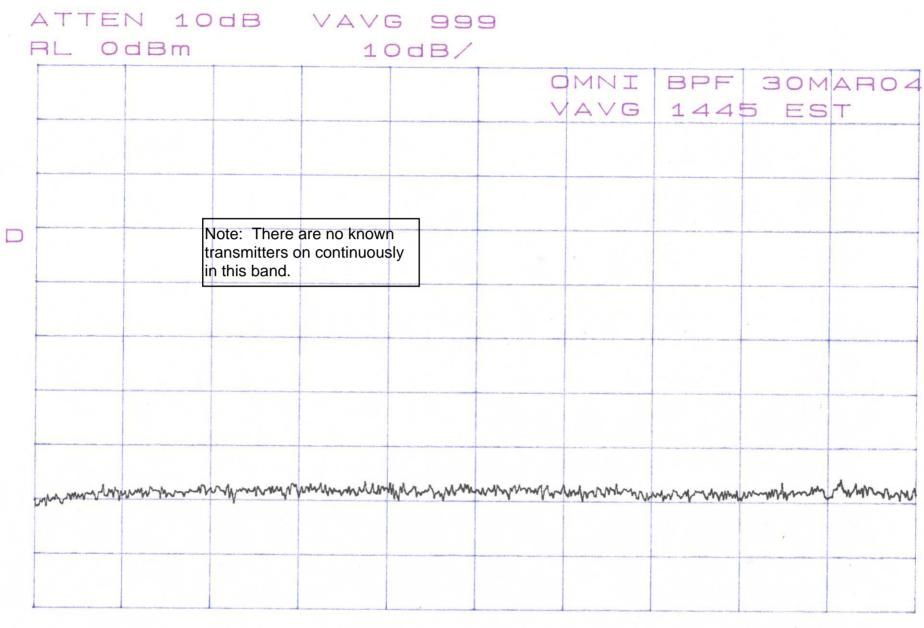
CENTER 128.000MHz SP \*RBW 10KHz \*VBW 10KHz
